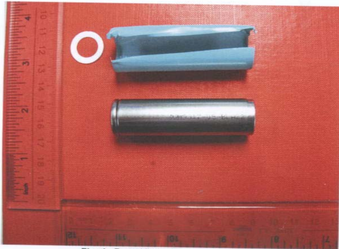
Fig. 4- Front View of remove insulation
